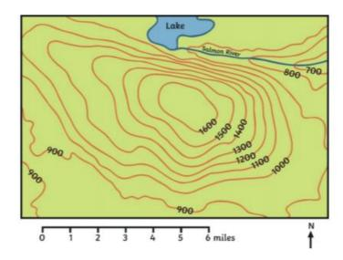
The closer the lines are together, the steeper the slope.
